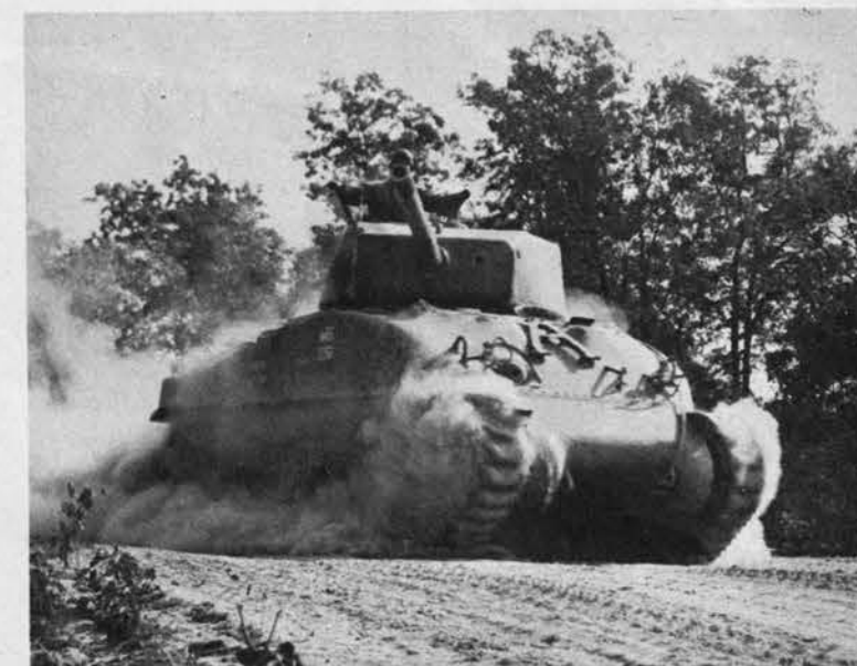
Third variation in the M-4's armament is a long-barreled 76-mm. cannon with extremely high muzzle velocity. It is supported by a heavy, rectangular gun mantlet. The turret is marked by an overhang at rear.
